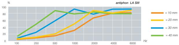
Above, in the graph, is an example of how the sound damping properties of one of our sound absorbing foams, antiphon® LA SIII, varies with thickness and frequency. This sound absorbing material is specially developed to comply with demands for fire resistance. This specific foam complies with the requirements in UL 94 HF-1. The National Fire Protection Association (NFPA) requires that all material in office machinery should comply with these requirements.
